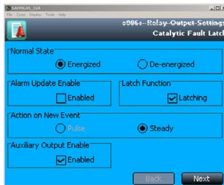
Figure 39. Fault Latch Output Configuration
