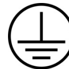
Figure 4. Equipment Earth (Ground) Point
