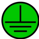
Figure 3. Protective Earth (Ground) Point
